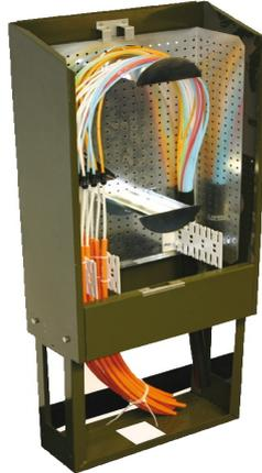
The FTTH Streetside Cabinet is a distribution/drop off access point within a blown fibre network. The cabinet allows a blown fibre cable of up to 24 tubes to be connected and distributed to up to 24 single tube blown cables. The cabinet is lockable to prevent unwanted access.
