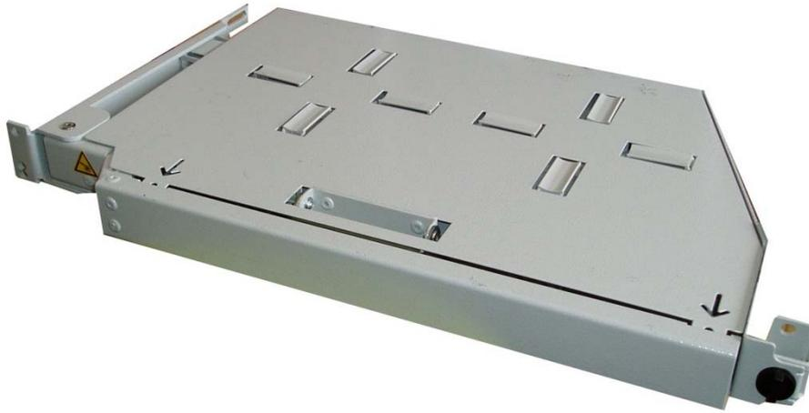
The POS is a 1U left-hand pivoting shelf, suitable for mounting into 19" racks and cabinets. The shelf can store up to 18 meters of 5mm tube/cable in 3 metallic trays . Up to nine 5mm OD tubes or cables and one 11.5mm cable can be installed into the shelf.
