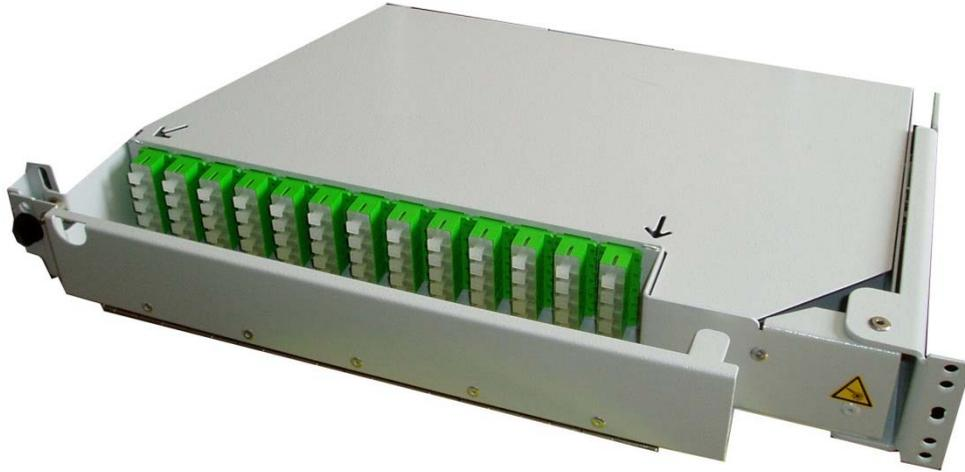
The MEC64 is a 1.5U Pivoting shelf, suitable for mounting into 19" racks and street cabinets. The shelf can accommodate one 1/64 or two 1x32 pre-terminated splitters. The shelf is supplied with SC/APC adapters and splitters pre-installed.
