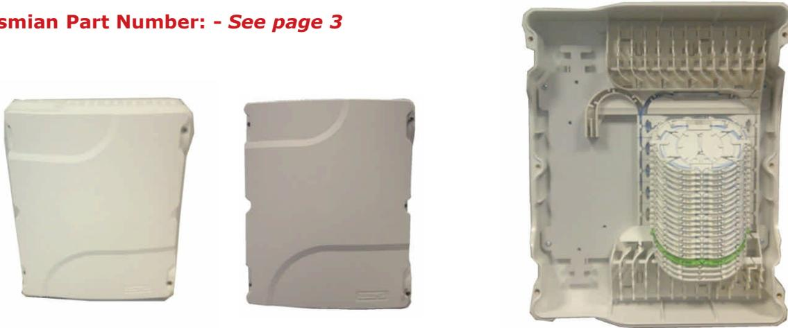
The 32 Way Splitter Node is a wall mounted product used for the distribution of fibres to customer drop cables. The unit can accommodate input cables (butt or in-line) for connection to a 32 way splitter device. Up to 32 drop cables of 3-6mm in diameter can be spliced to the output splitter legs and distributed from the box. Drop cable ports are provided on both top and bottom faces of the box and top and bottom manifolds provide easy routing of fibres within the unit.
